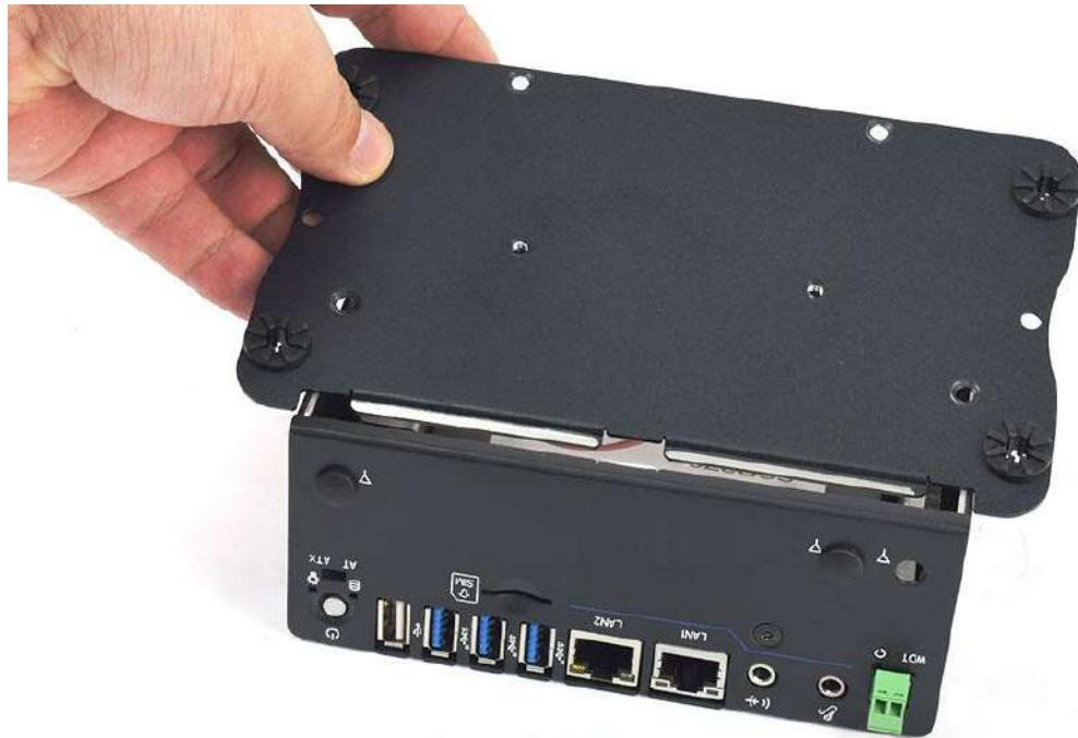
2. Lock the bottom cover with the four screws.
