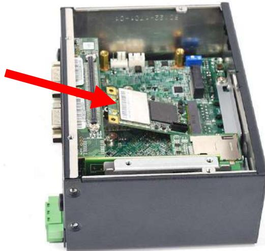
2. Press the mini PCIe card or mSATA module down and lock it with two screws.
