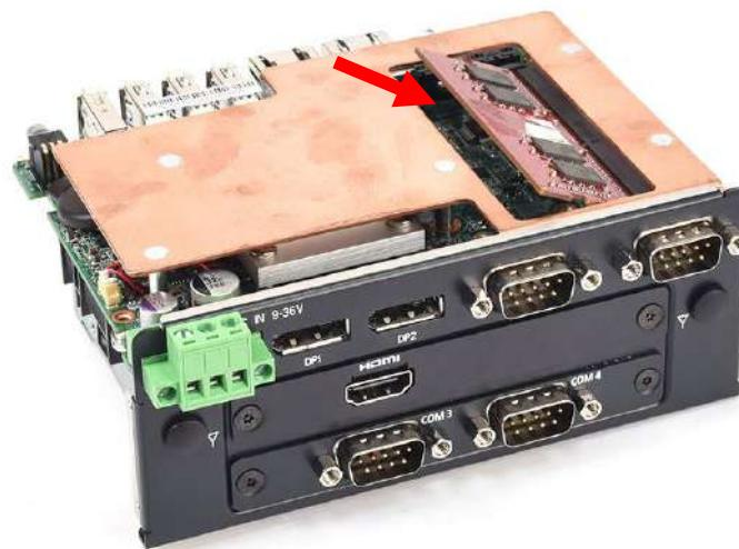
5. Press the memory module vertically downward until you hear the “click” sound. Make sure the memory module is firmly in place.
