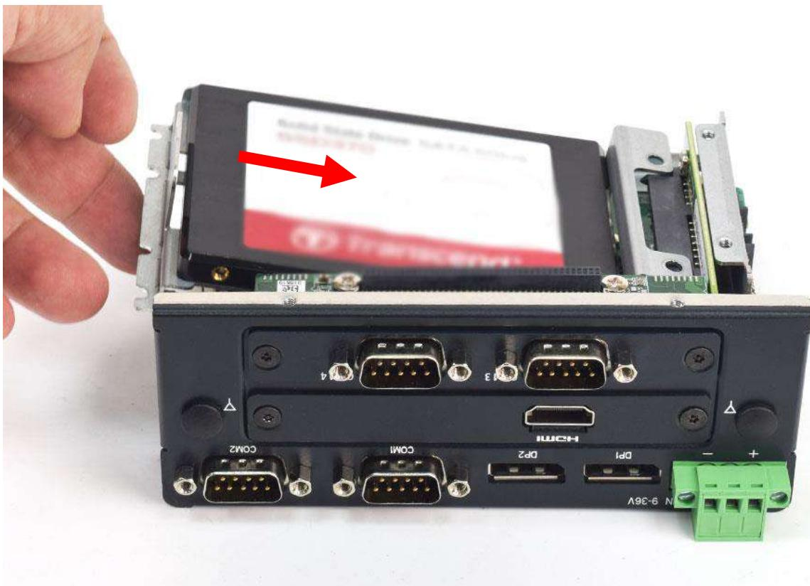
4. Fasten the four screws to lock the HDD bracket in place.
