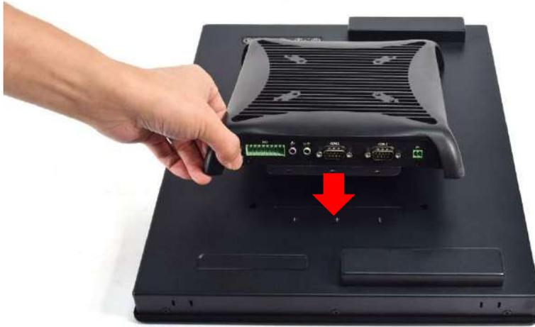
2. Ensure the PC Module is aligned with the VIO Display Module and push it down gently.
