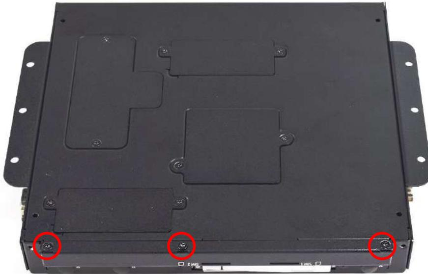
2. Remove 4 screws located at the front and side face of the system as pictured below. The screw locations are highlighted in red.
