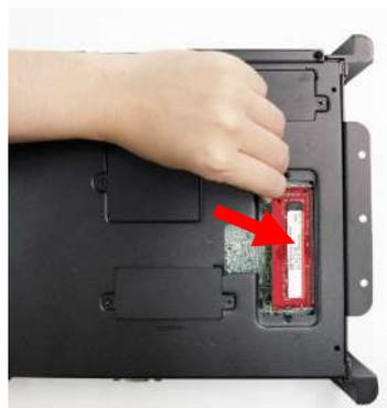
3. Press the memory card down until you hear a click. Ensure the memory card is secure before replacing the cover.
