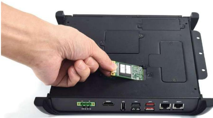
3. Press the mini PCIe card or mSATA module down and ensure it is secure before screwing the cover back on.
