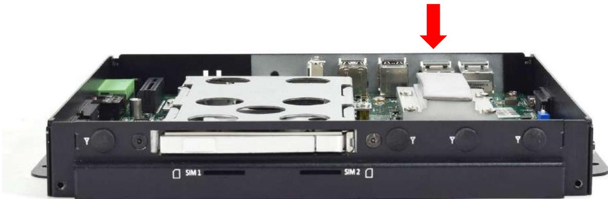
2. Close the chassis top cover following the below direction and make sure the aluminum part on the top cover is touching the thermal pad on CPU thermal block.
