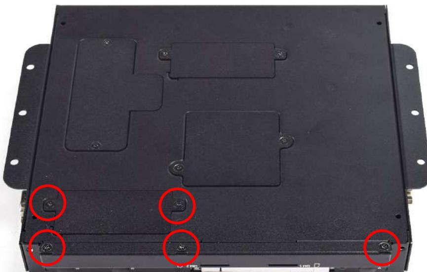
7. Fasten the 4 screws located at the front and side face of the system as pictured below. The screw locations are highlighted in red.
