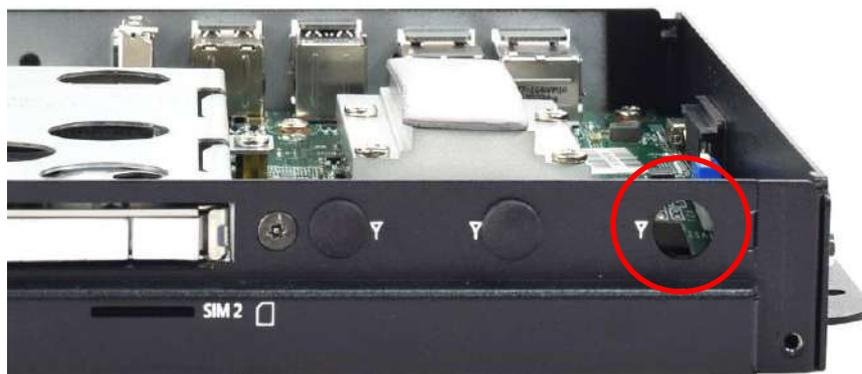
4. Pass the RF connector at the end of the cable around the gap between the iron piece and the motherboard and connect it to the communication module.
