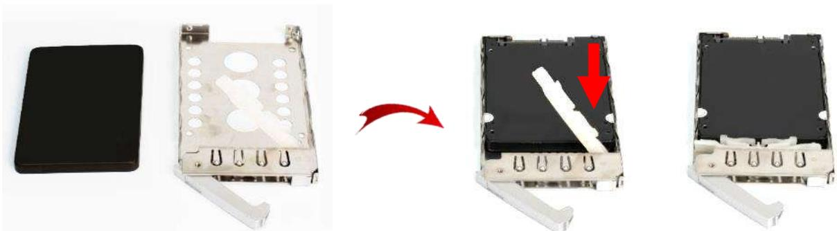
4. Place the tray back into the bay and ensure the tray lock is secured.
