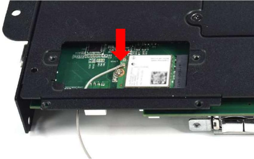
5. Put on washer and fasten the nut with antenna jack as indicated below.
