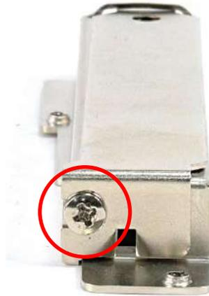
5. Attach the PCIe expansion card and then fasten the screw in the circle indicated below.
