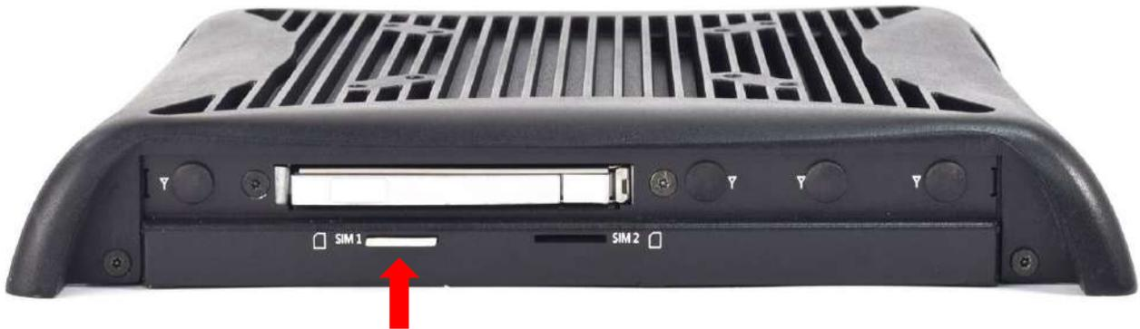
3. Please refer to the table below to note which SIM slot to insert your SIM card into according to the matching Mini PCIe type.
