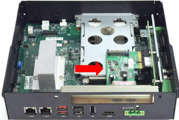
7. Ensure the gold fingers are inserted properly into the slot.
