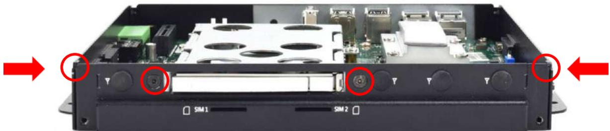
3. Remove antenna hole cover on the system panel as indicated below.
