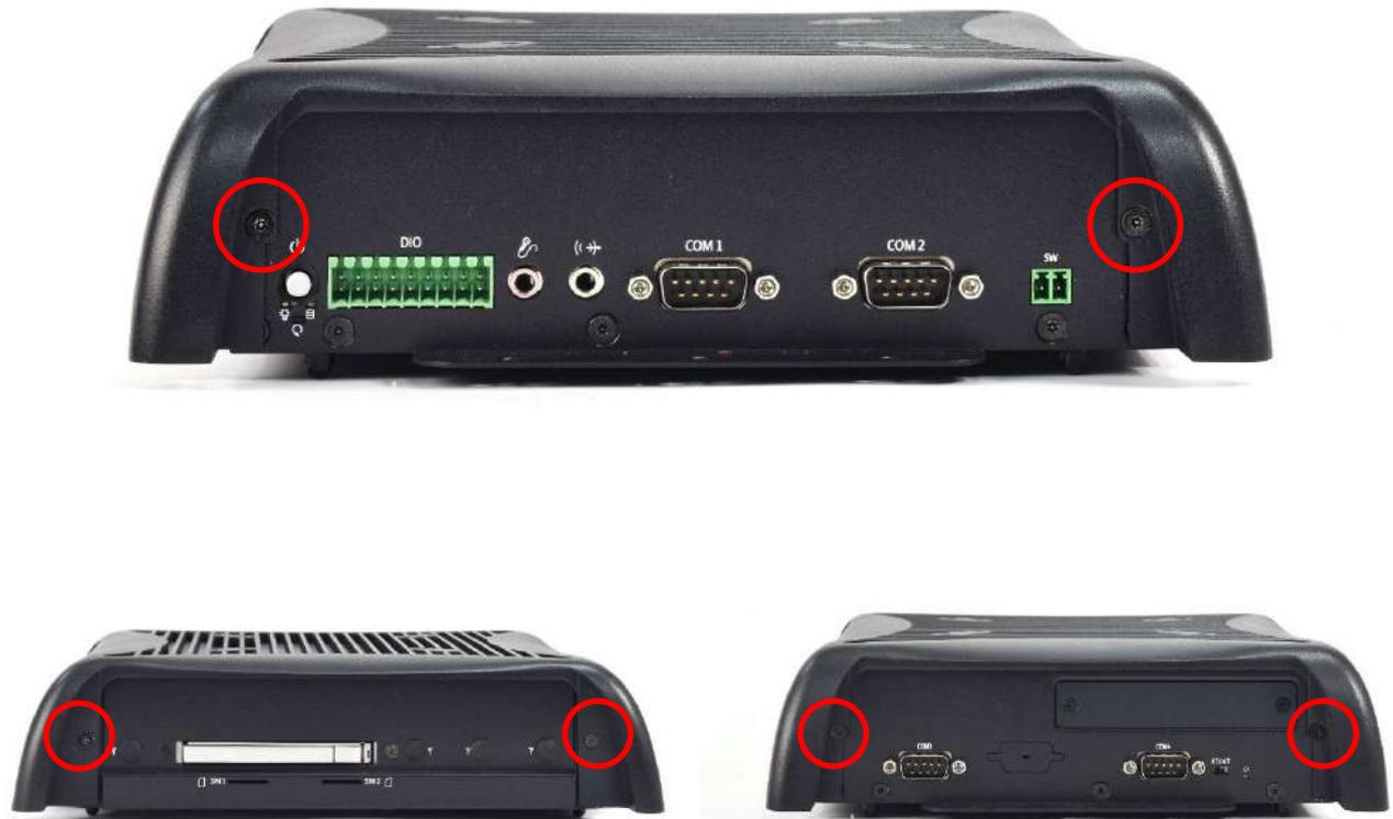
2. Once unscrewed, remove the top cover of PC module as shown below.
