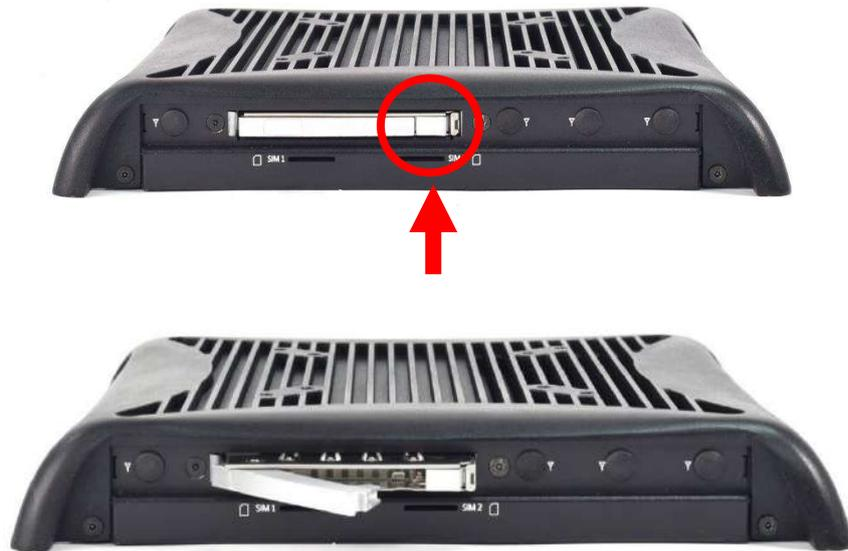
2. Unlock the drive lock by lifting the plastic insert up, then insert the HDD/SSD card.
